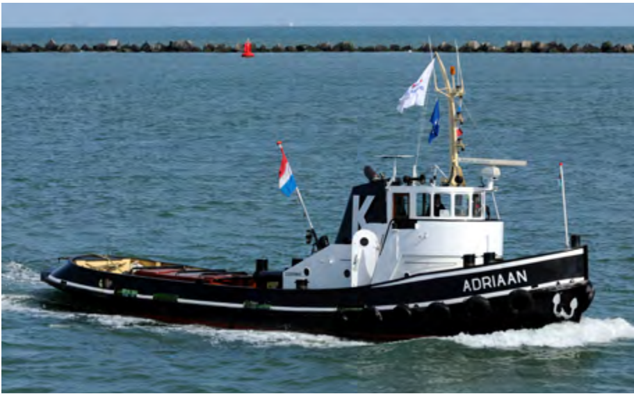
ADRIAAN was built in 1957 by Wortelboer, Gouderak, for account of Adriaan Kooren. 380 bhp Stork-Ricardo main engine. Operated mainly on dredging projects in The Netherlands, France and Germany. For many years operating in support of the Easterscheldt storm surge barrier construction as well as the construction of the Maeslant storm surge barrier. In 1986 transferred to Kooren International and used as a harbour / shiphandling tug. Still owned by Kotug she is now registered as maritime heritage. Part of the Maasluis Tugboat Port fleet she is maintained in top condition. Seen here in use as an operational museum tug photo: Hans Hoffmann
