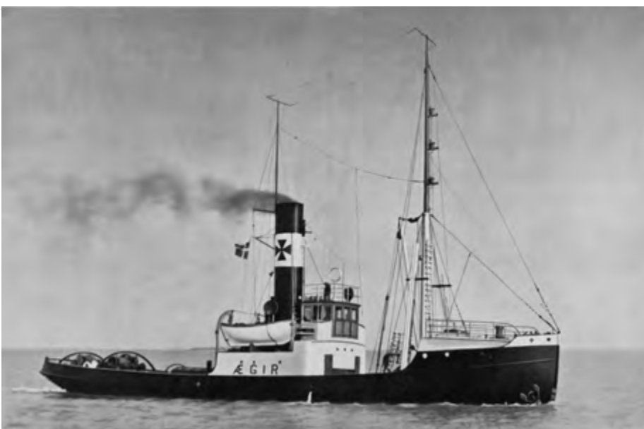
AEGIR - a 1906 built salvage steamer for account of Svitzer. The 365 ihp was built by Kobenhavn Flydedok. 1943 modernised and re-engined. Scrapped in 1955. AEGIR was the first 'foreign' salvage vessel to arrive in Poland post WW2 to help clear the ports (see also TugZine 33)
