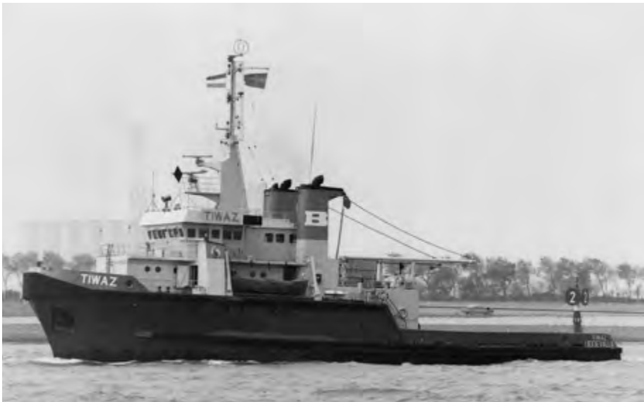
TIWAZ - Bohus Tugs - Built 1978. 43,39 x 12,23 m. 7.040 bhp / 85 ttp. 1986 sold to Bahmscan Towing & Salvage, Bahamas, as SCAN FORCE. 1989 to Bukser og Bjergning as BOB. 1991 BOA FORCE. 1994. Collided and sank, raised and scuttled 5.000 m of water near Thevenard Island
