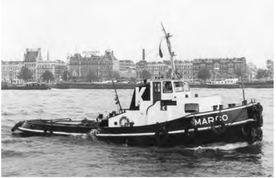
MARCO was a 1954 newbuild from shipyard Bijlsma, Wartena. 17,20 x 4,55 m. Draught 2,10 m. 220 bhp Caterpillar. Seen here at Rotterdam 27-11-1975. 1983 sold to L.J. van de Geer, Spijkenisse. Same name. Almost immediately resold to Scheffer Salvage, Urk, renamed ARGO photo: Frits van der Hoek
