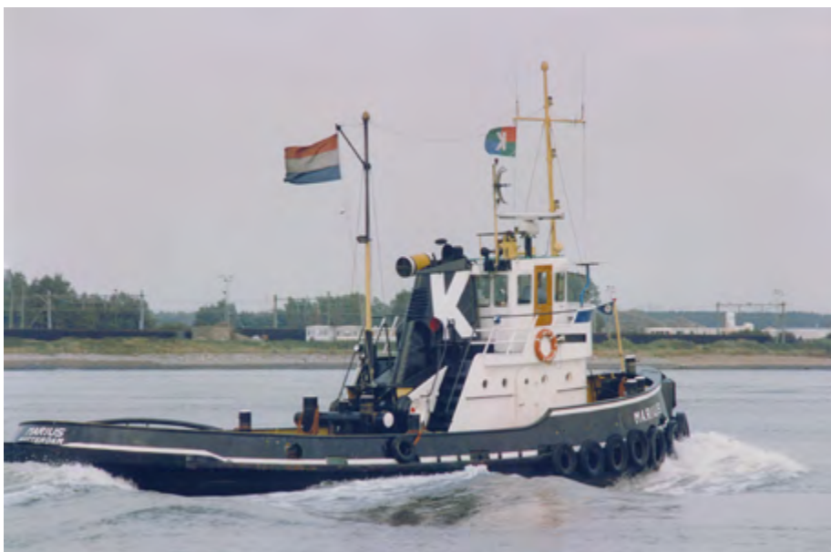
MARIUS seen here in 1972 - was built in 1962 by Shipyard Paans, Roodevaart (yn 237). 21,50 x 5,80 m. draught 2,35 m. Main engine 510 bhp Stork-Ricardo replaced in 1980 by 860 bhp Stork. 10 tpb. 1980 modernised by Van de Sande shipyard, Breskens. This was A. Kooren's first seagoing / coastal tug. 1986 to Kooren International. Mainly employed in civil engineering and occasionally as a shiphandling tug at Rotterdam. She has been active on projects far away from her home port Rotterdam. .1996 sold to A. Kaptein & Zn Duwsleepvaart, Urk. Renamed COBY . 2018 sold to Treffers Scrapyard, Haarlem. Same name photo: Job van Eijk
