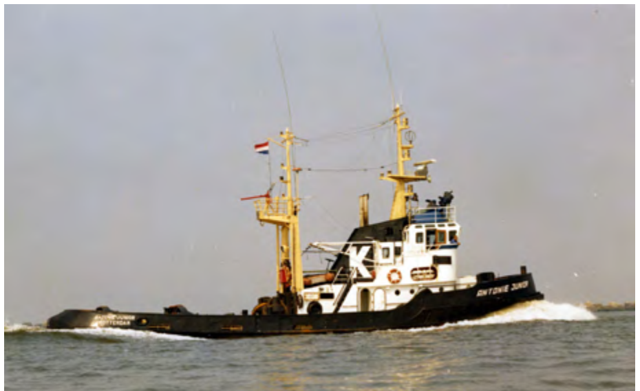
ANTONIE JUNIOR was built by Kramer & Booy, Kootstertille, for account of Adriaan Kooren. The 1.320 bhp 21 tpb tug was designed for deepsea work as well as for use on hydraulic engineering projects. In 1988 transferred to Kooren International. 30-12-1996 to Engelsman, Makkum. Same name. 2002 sold to Remolcatuna (Tom Juijn) for use in the tuna industry. Renamed ANTONIE and based at Cartagena. 2004 renamed ANTONIE X. 12-2013 sunk off the North African coast. It is of interest to note that the two main engines originate from the tug VIKINGBANK which was lost during a salvage attempt off Hoek van Holland, raised and later sank again when the lifting gear of the sheerlegs broke. Again raised and demolished but the engines were overhauled and purchased by Kooren photo: coll. Job van Eijk
