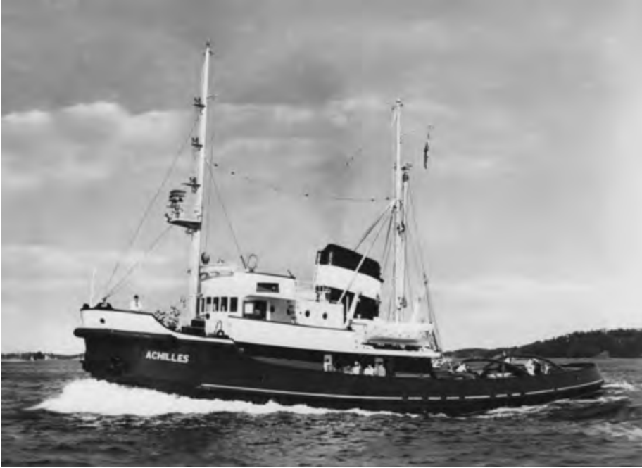
ACHILLES was built in 1962 by Handel & Scheepsbouw Maatschappij Kramer & Booy, Kootstertille, The Netherlands. Dimensions 32,73 x 8,62 x 4,11 m. Main engine Ruston & Hornsby 9 AT CM delivering 2.050 hp postcard: issued by Norsk Bjergning- och Dykeri
