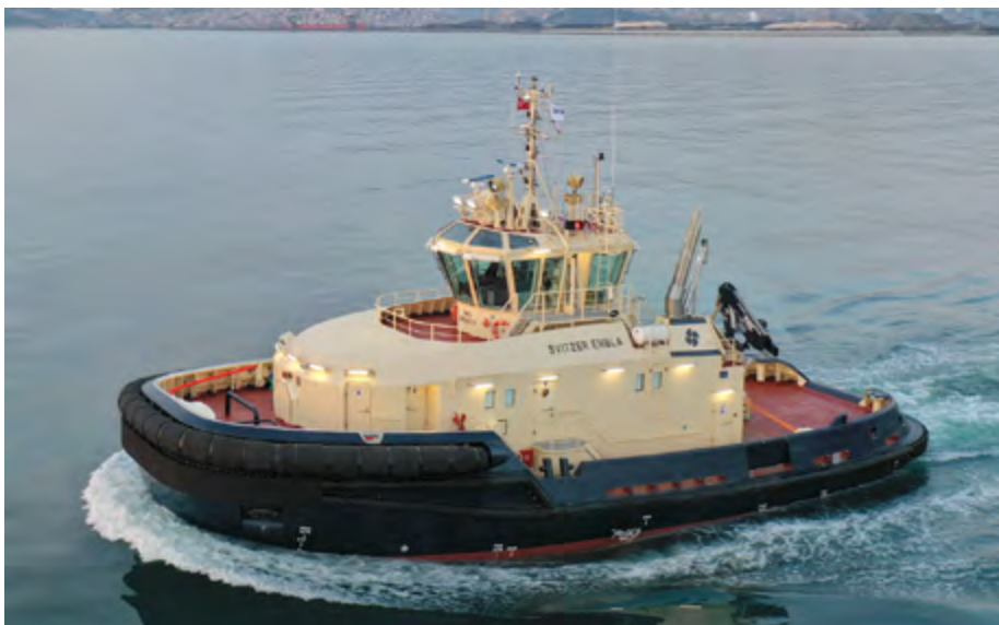
SVITZER EMBLA. Built 2021 by Med Marine's Eregli yard in Turkey. 30 x 12,6 m. M.A.N. Energy Solutions, 4.080 kW. Tug was designed by Robert Allan for shiphandling and icebreaking in the Göta River and Trollhattan Canal
