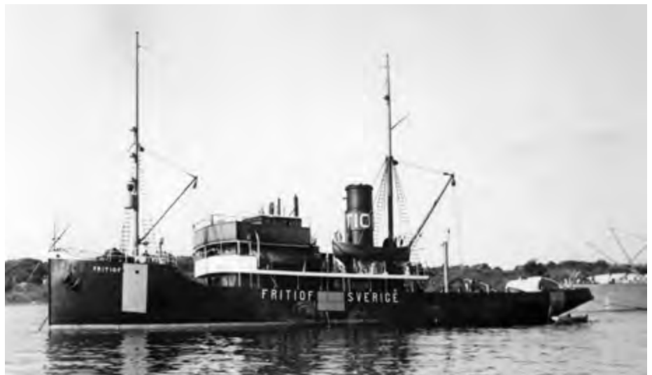
FRITHIOF - Göteborg Bogsering - prior to her sale to Svitzer. Built 1921 by AB Götaverken, Göteborg. Dimensions 51,06 x 10,55 x 4,25 m. Main engines 2x Burmeister & Wain 6-cyl. total output 1.220 hp. In 1956 re-engined with 2x MaK 6-cyl. total output 2.300 hp. Renamed Em. Z. SVITZER which was altered to SVITZER in 1958. She survived until 1974 when she was broken up in Spain photo: coll. Job van Eijk
