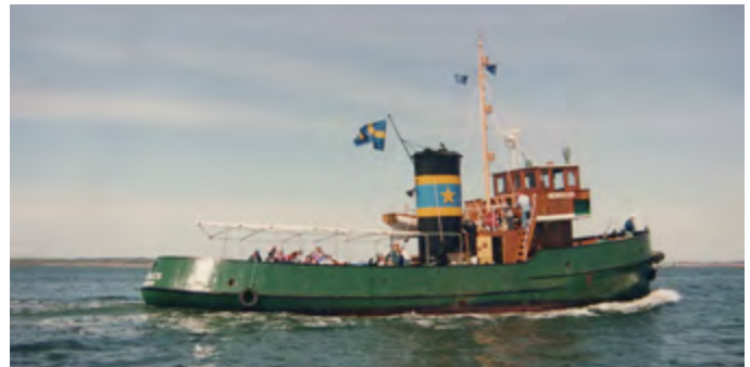
HERKULES (1939 – 24,43 x 6,21 m – 650 bhp) was built for C.L. Hanssons Stuveri AB. 1983 Johnson Bogser AB Marin Service AB, same name. 1985 to Föreningen Bogserbaten Herkules. Refurbished by the society and in 1989 donated for use as a museum tug
