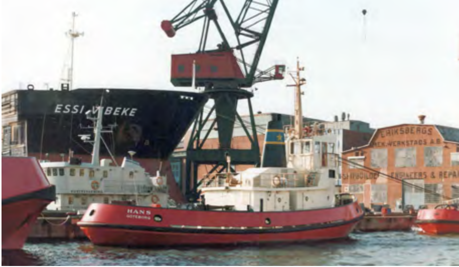
HANS- Johnson Line. Built 1967 for Rödabolaget. 25,00 (oa) x 8,50 (mld) m. 2.87- bhp - 28,5 ttp. 1992 sold to Oskarshamn s Hamn AB as HERBERT
