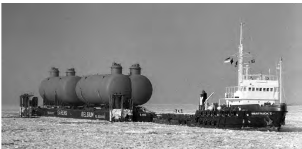
SEATRUCK 1 is the former tug / supply vessel ADAMSTURM owned by VTG Hansa (Offshore Supply Association). She was built in 1968 by J.G. Hitzler (yn 700). Dimensions 53,47 (oa) x 11,02 (oa) x 3,97 m. Draught 3,55 m. Main engines 2x 16-cyl .M.A.N. total output 2.740 bhp. Bollard pull 34 tonnes. Acquired by Adriaan Kooren in 1986. 1 January, 1988, transferred to Kooren International. 1990 sold to Venus Trading, London, renamed SAFE CARRIER . 1998 sold, owner unknown, as DESTINEE . 2011 sold, renamed SIMONE , registered at Sao Tomé. No further details photo: coll. Job van Eijk.
