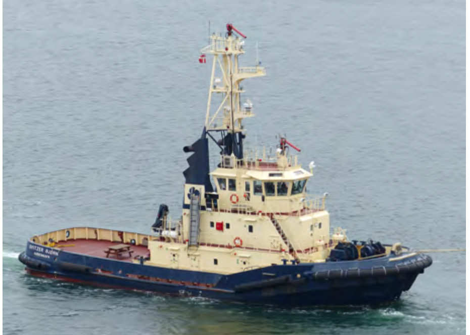
SVITZER BJÖRN, ex BJÖRN operated by Rödabolaget. This is one of a series of three stern drive tugs acquired in Japan. Built 1991 for Rödabolaget. 32,89 (oa) x 10,23 m. 3.950 bhp./ 54 ttp. Reverse tractor with Kawasaki Rexpellers. Sisters JOHN and LARS photo: Ko Rusman
