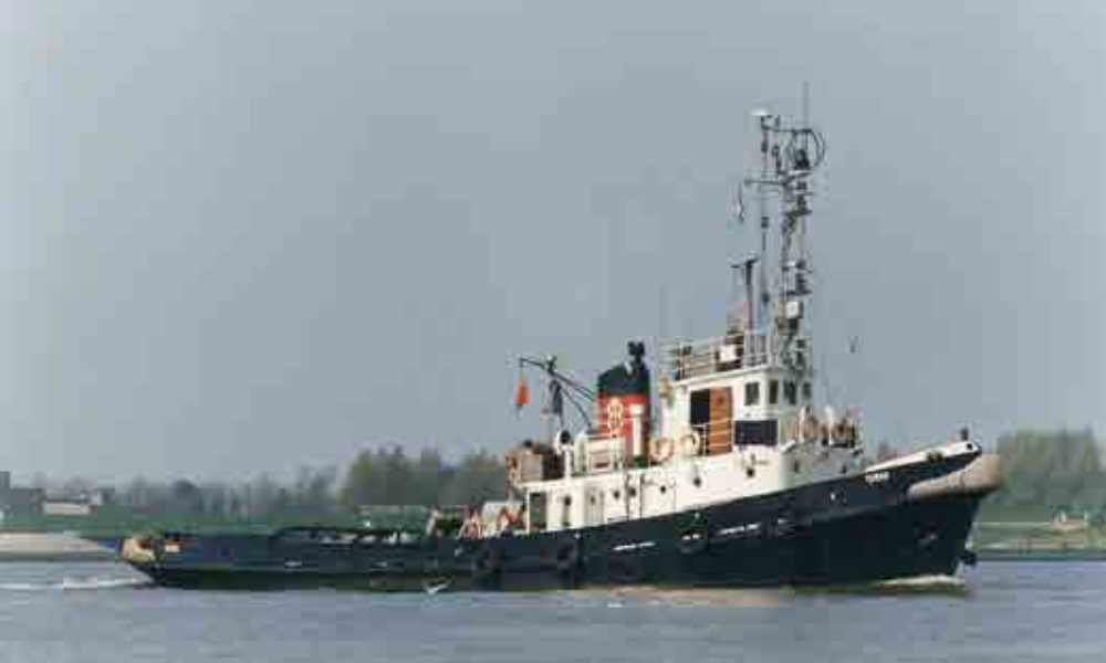
TUMAK (pictured in the Rotterdam Waterway) and sister ROSOMAK were the first newbuilds ordered for PRO. The design incorporated the double use as tug and rescue vessel / salvage tug photo: coll. Job van Eijk
