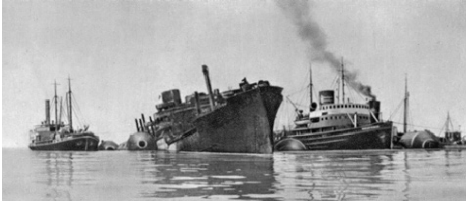
Wreck clearing: salvage of SEEBURG. Raised from the bottom with the aid of 'camels' being prepared for transport. On the left SMOK, on the right the icebreaker / tug SWIATOWID
