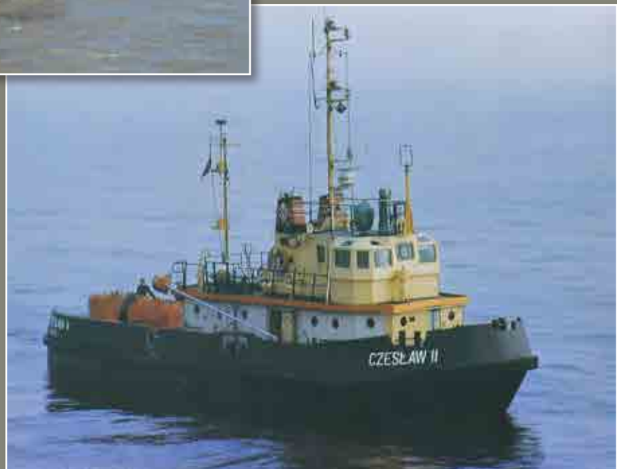
CZESLAW II is a former tug that was reconstructed as a pollution-control vessel photo: Polish Ship Salvage Co
