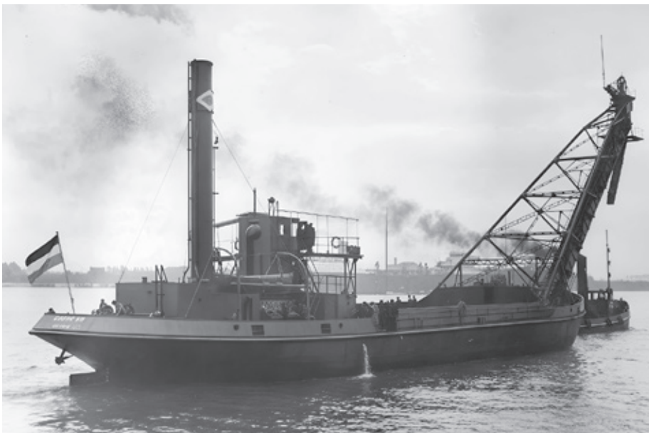
ROBUR VII seen here was a coaling vessel built in the Netherlands by Gusto. She was certified for bunkering operations in the roads. The vessel was fitted with a huge transporter boom on the bow to deliver coal into the bunkers of steamers. Carrying capacity was 1.000 tonnes, discharge rate 400 t/hr. A conveyor belt ran along the hold up to the top of the transporter boom from which the coal was dumped – via a chute – into a ship's bunkers. During WW2 converted to a salvage vessel and ultimately - via Zegluga Polska - ending up with Polish Ship Salvage photo: Digital Collection Shipyard Gusto Heritage Foundation
