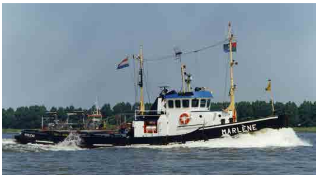
Adriaan Kooren's MARLENE - 570 bhp 8 ttp - was used as a shiphandling tug during the start-up period
