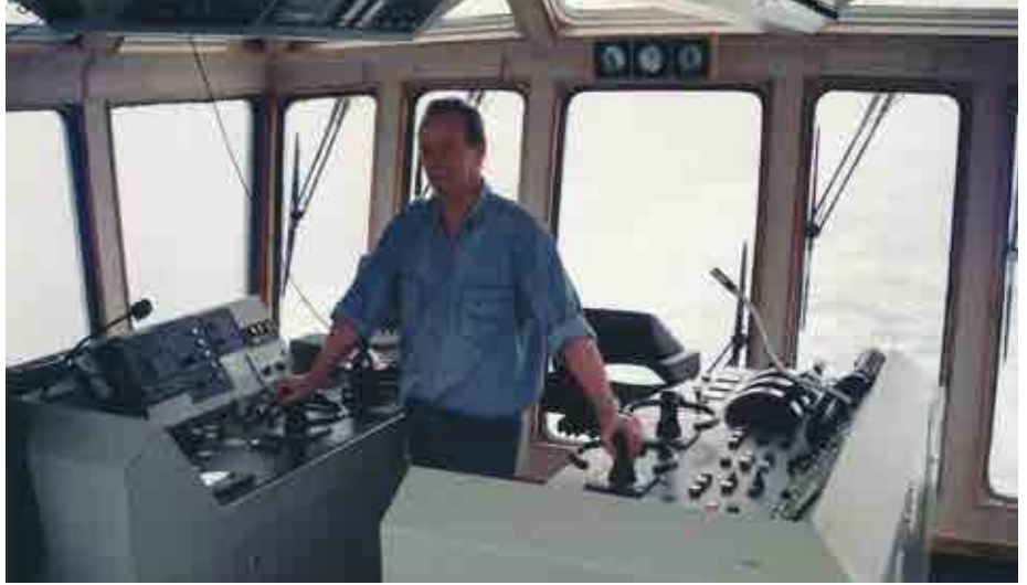
Captain Aalbers steering RT PIONEER with the two forward controls. The aft control is in the centre position
