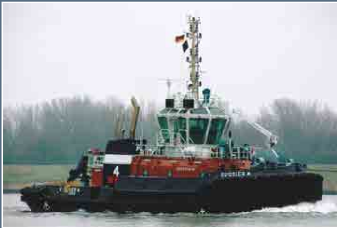
The Rotor Tug BUGSIER 4 was built in 2008 by ASL. 6.529 bhp - 86 tbp photo: Sjaak van der Meer
