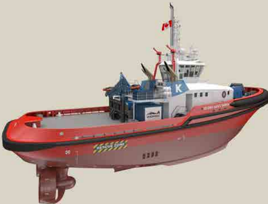
Artist's impression of the dual fuel methanol-diesel stern drive for Canada artwork: courtesy Robert Allan Ltd
