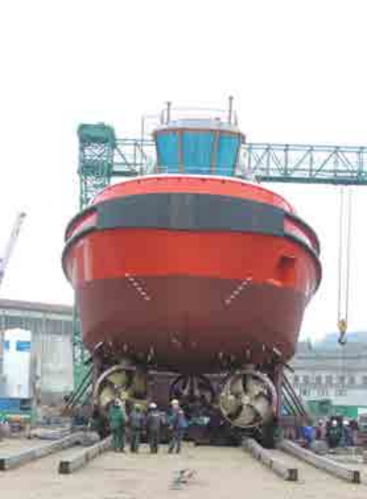
Visible are the spousons, lack of docking struts, the position of the 3 schottel thrusters
