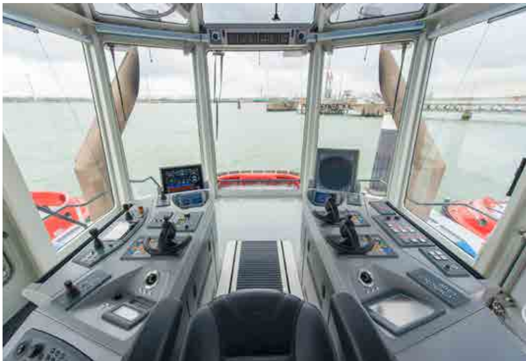
The Alphabridge Tugboat Console on RT EVOLUTION - also note the almost unobstructed all-round view
