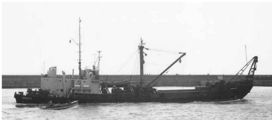
TOPMAST 18 was a reconstructed landing craft adapted for salvage and cargo recovery
