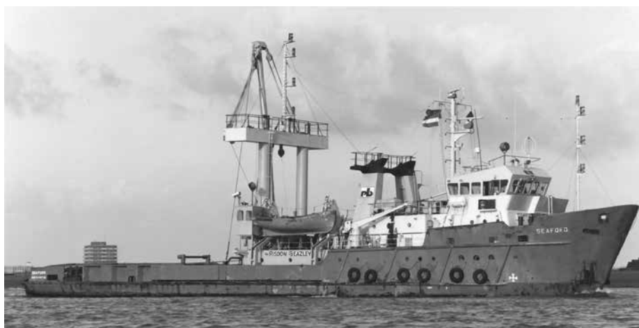
SEAFORD was a former tug / supply vessel adapted for searching for wrecks in deep water
