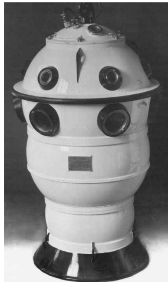
Galeazzi brand observation chamber - designed for 550 m water depth photo: coll. Job van Eijk
