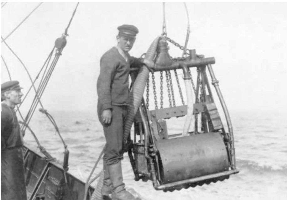
P.A. van Hecking Colenbrander with his improved coal grab with water injection - on board STORTEMELK in 1924
