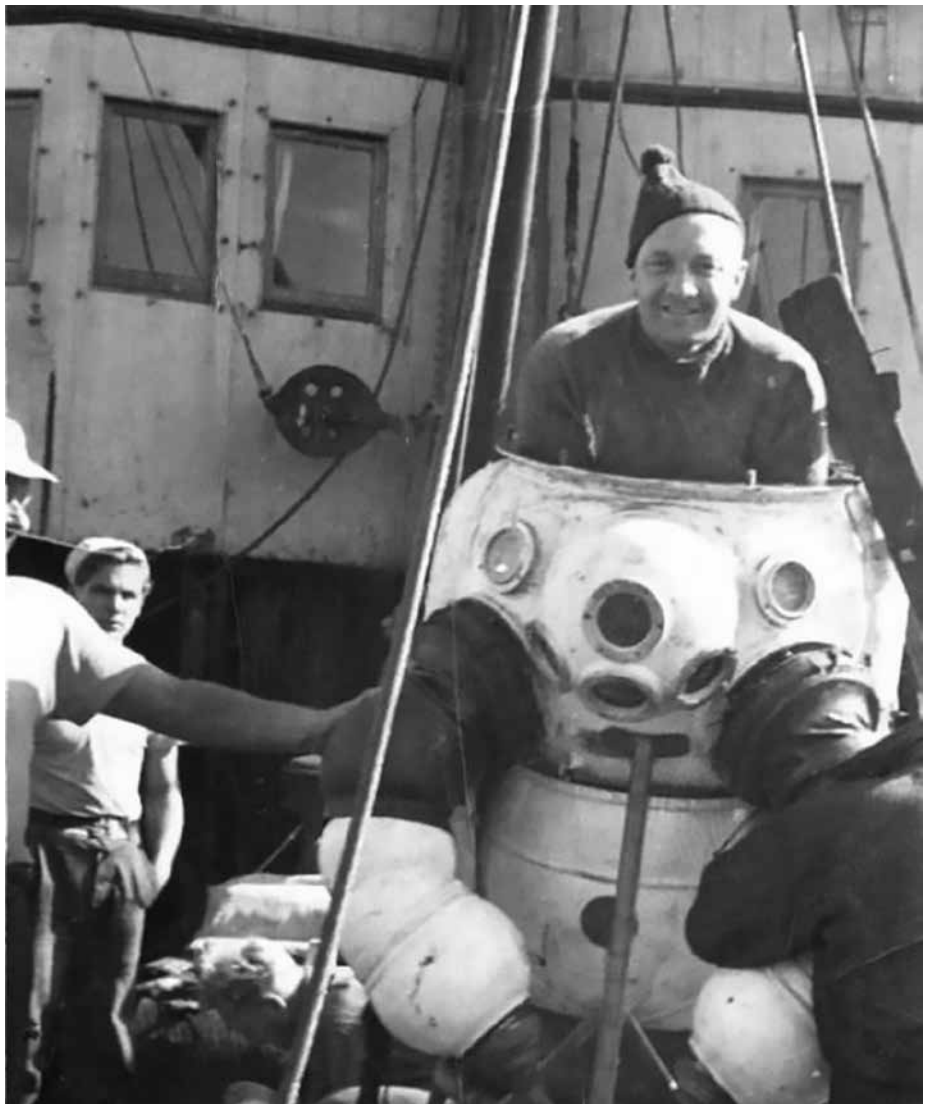
An ‘iron man’ diving suit used on the NIAGARA recovery operation. Variations of this have been used since before EGYPT. In general the salvors found these suits too cumbersome and preferred the option of the observation chamber in many cases photo: coll. Whangarei Museum
