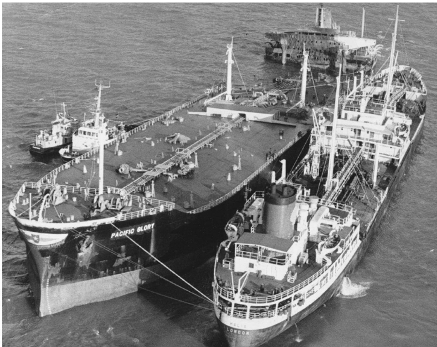
The tanker PACIFIC GLORY in 1970 October 1970 collided, started sinking and caught fire. The tanker was moved to a sandbank to avoid a possible total loss. The fire was extinguished but the tanker could not be freed by the tugs. The lightering tanker HALIA operated by Shell U.K. was chartered for a ship-to-ship transfer (STS) operation. After lightering the casualty was refloated and towed to a shipyard for repair. In this photo the STS is ongoing. To recover 18.000 tons of oil 7 days of fair weather were needed. Barely visible alongside is the Smit (NRS) tug SMITHBANK
