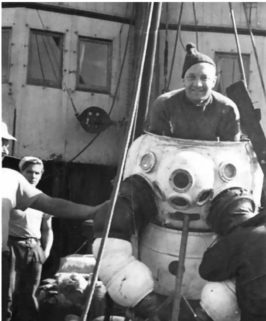
An ‘iron man’ diving suit used on the NIAGARA recovery operation. Variations of this have been used since before EGYPT. In general the salvors found these suits too cumbersome and preferred the option of the observation chamber in many cases photo: coll. Whangarei Museum
