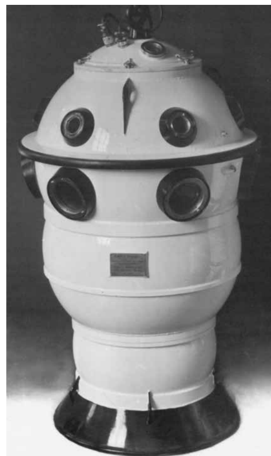
Galeazzi brand observation chamber - designed for 550 m water depth
