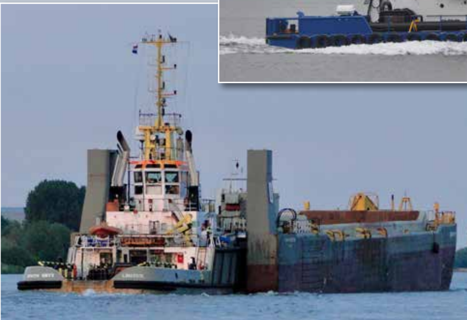
The tug UNION ONYX is seen here in the Oude Maas en route IJmuiden to Moerdijk on 12 May, 2024. The tug was constructed for account of the Belgian U.R.S. - a Smit subsidiary - as a seagoing / coastal tug but on take-over of Smit by Boskalis reconstructed as a 'pin' boat for mating with barges involved in dredging operations. Here she is pushing the barge TERRAFERRE 501 photo: Nico Giltay
