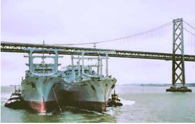
Departing Alameda with double tow; harbour tugs keeping the tow in line photo: coll. Kees Pronk
