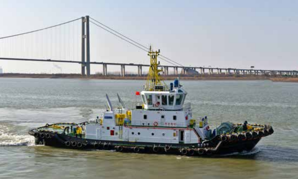
Jiangsu Zhenjiang recently delivered the first Chinese domestic hybrid diesel-electric tug - YONGGANG TUO 80 - to the owners Ningbo Oil Handling photo: Jiangsu Zhenjiang Shipyard
