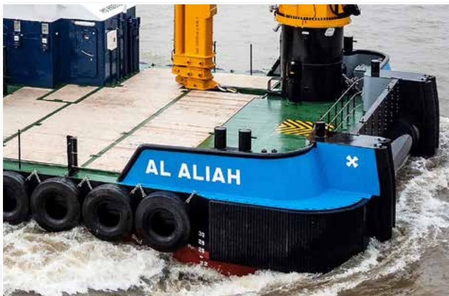
Bow and side fendering, push knees and bow roller photo: Kloet / courtesy Damen Shipyards
