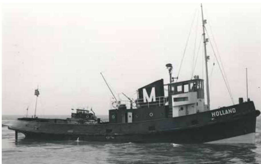
HOLLAND - ex CALAISIE , ex LAUENBURG , ex PORT DE BEYROUTH was purchased in 1961 - former 900 ihp steam tug. Reconstructed as motor tug by Terneuzensche Scheepsbouw in 1962. 1.170 hp. 1987 extensively rebuilt and re-engined - 1.600 bhp - 1991 sold to Jan Zwagerman - 1993 in lay-up, 1996 auctioned. Photo shows the tug in her first appearance as motor tug photo: J.W.F. Smallegange
