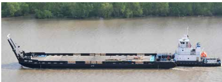
The DRIFT RIVER / ALULAQ combination is designed by Coastwise Engineering. Brice Marine uses the ATB to service remote rural Alaskan communities. The ATB is fitted with a Finnish Beacon pin system
