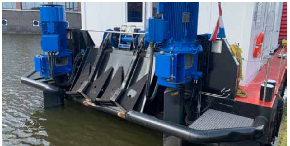
Hydromasters - one in the raised position, the other on in the lowered position, Anchors and anchor winch in between
