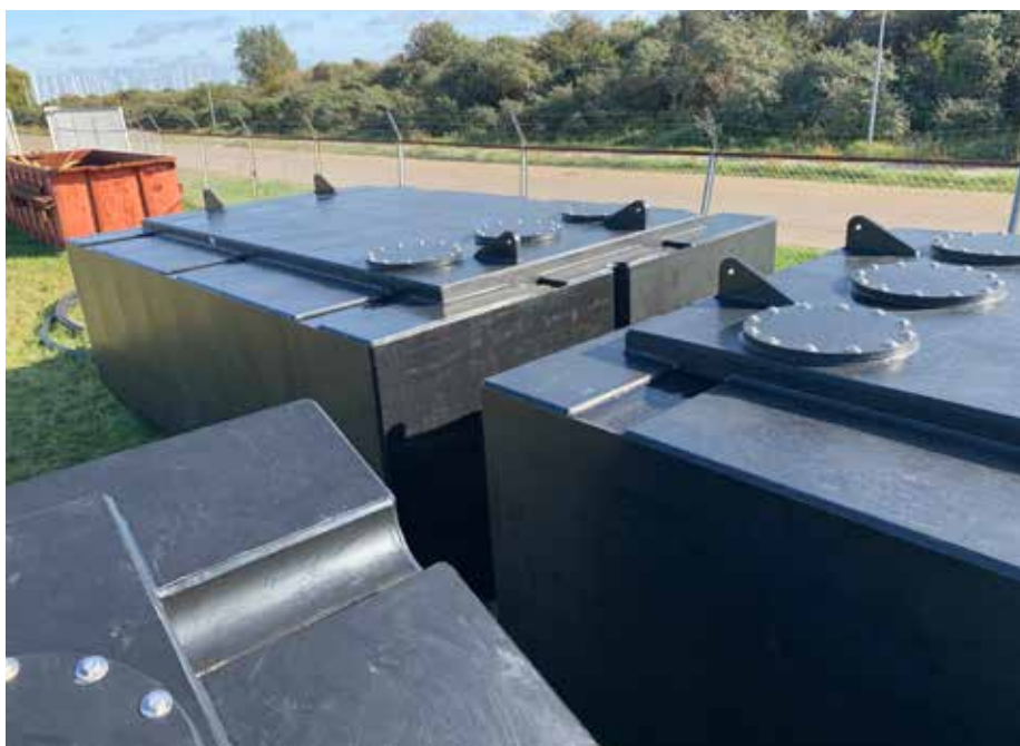
Hull cubes awaiting assembly
