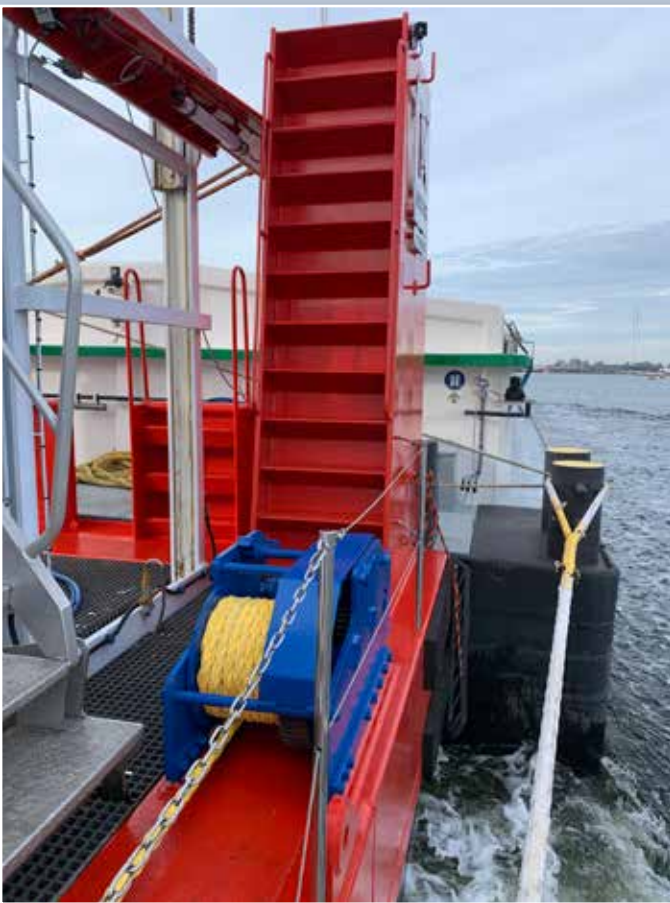
Kotug E-PUSHER 1 with barge. Note Kooiman coupler winch position photo: Kotug / Bas van Hoorn
