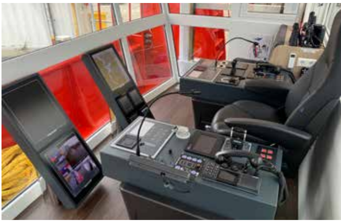
Wheelhouse. Nearest camera control desk with port side Hydromaster controls, nav lights, VHF and barge bow thruster control
