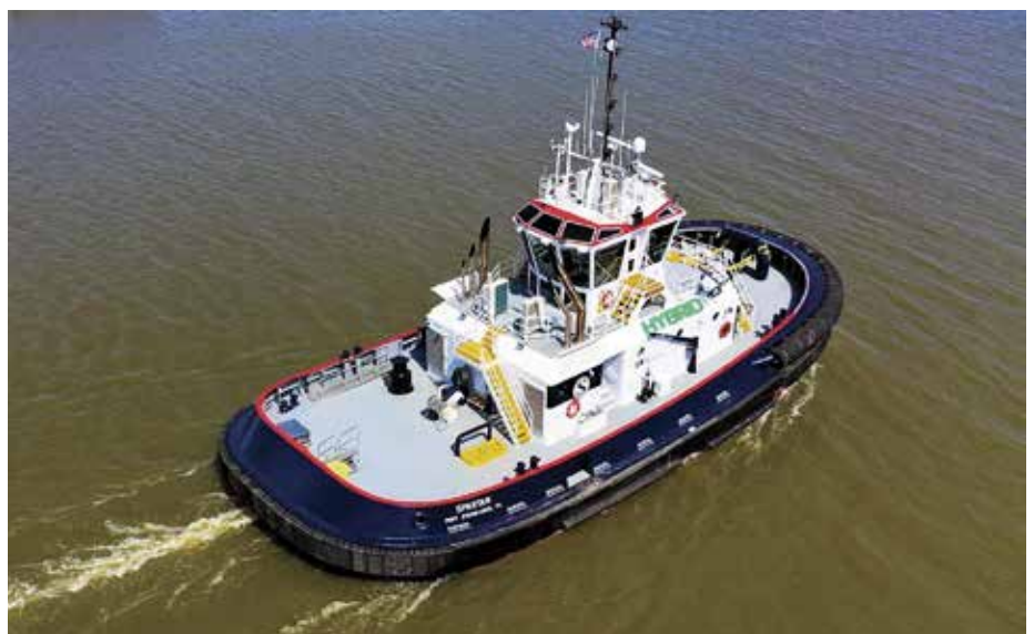
SPARTAN is one of two hybrid shiphandling tugs delivered to Seabulk Towing
