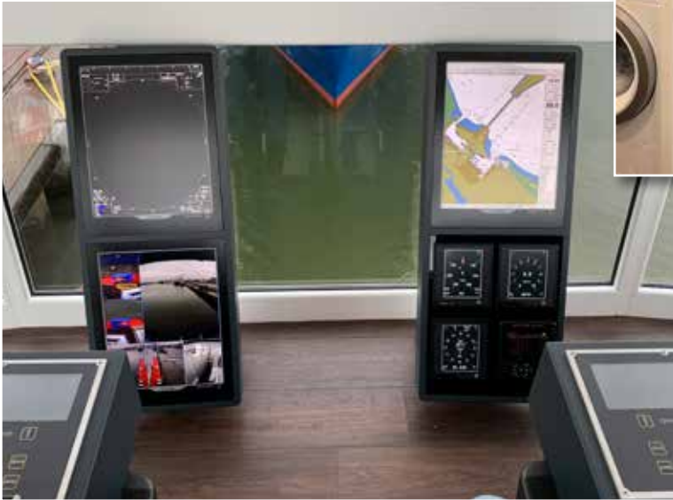
Helmsman's information displays: left radar and camera views, right position display, Rate-of-turn indicator, echosounder, wind speed / direction indicator photo: Kotug / Bas van Hoorn
