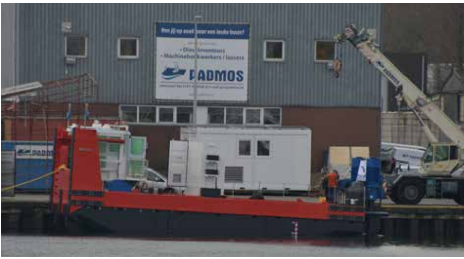
Part assembled hull alongside at Padmos. Switchboard container already on board photo: Ruud Zegwaard
