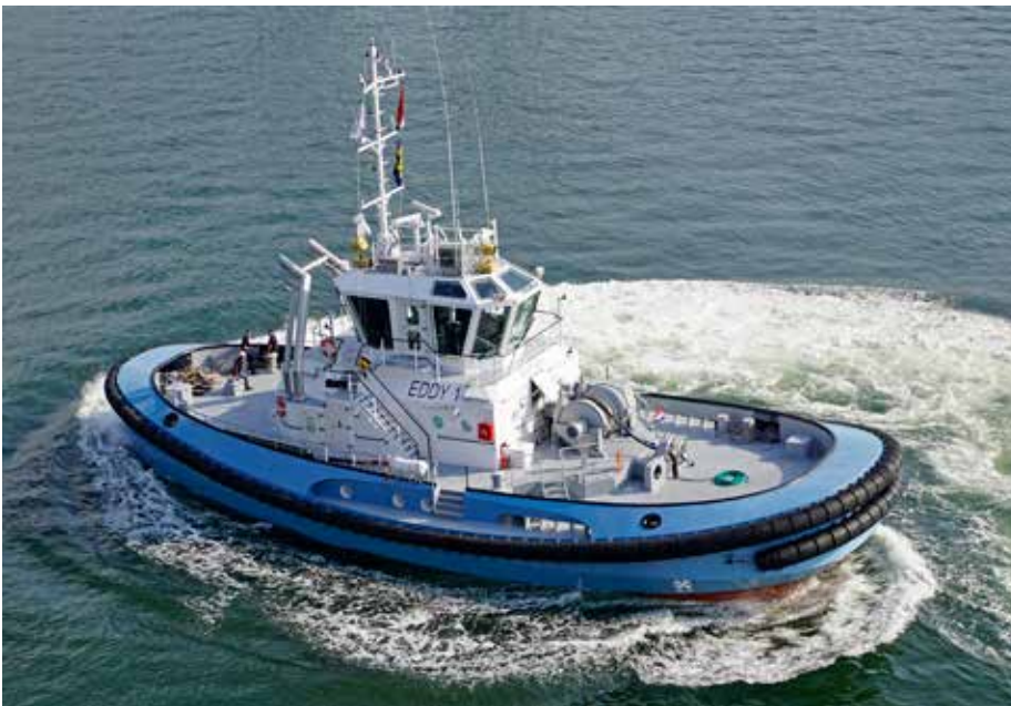
EDDY 1 seen here on 18-09-2014 was built by Holland Shipyards. The tug has the drives in-line forward and aft. Tested around the globe she got a charter with Iskes Towage as ATLAS. Currently operated in Norway as FFS ATHOS
