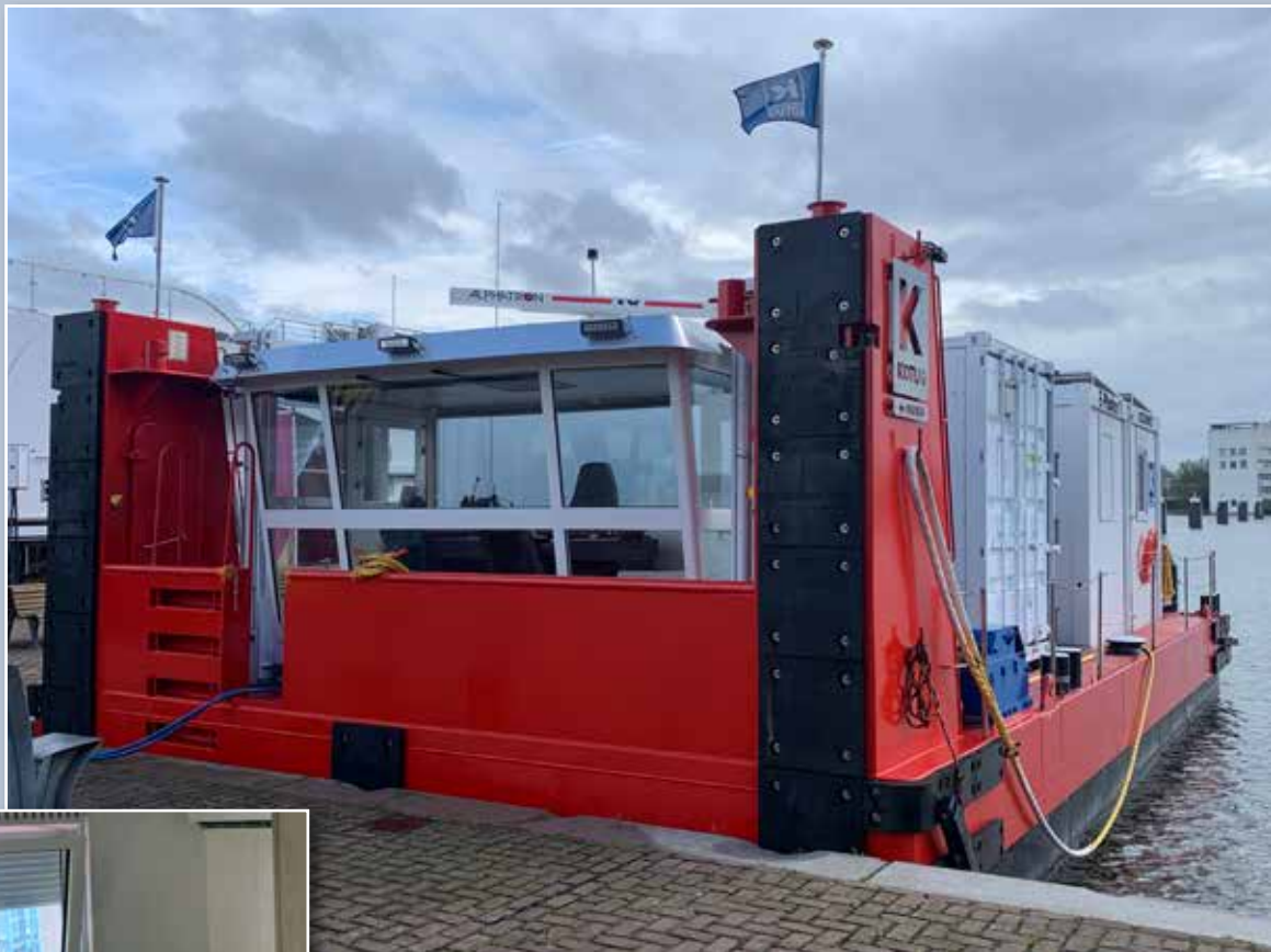
Kotug E-PUSHER 1 with barge. Note Kooiman coupler winch position photo: Kotug / Bas van Hoorn
