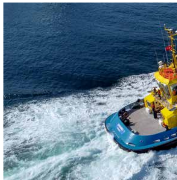
The two SAAM-ordered electric tugs are about to be delivered by Sanmar. Battery power is 3.616 kW delivering 70 tons of bollard pull. DYNAMO
