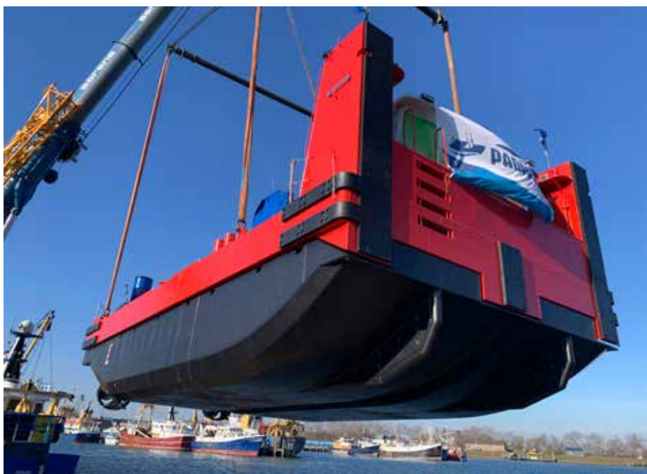
Hull and frame mated, wheelhouse installed
