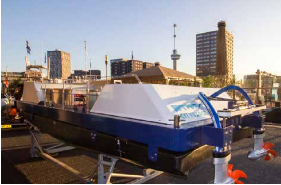
Kotug CITY BARGE ONE ashore showing propulsion pods
