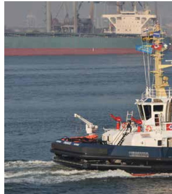
FREGATE - seen here on 9-05-2018 running trials - is a combination shiphandling tug and a water injection dredging 'plough' hanging from the stern
