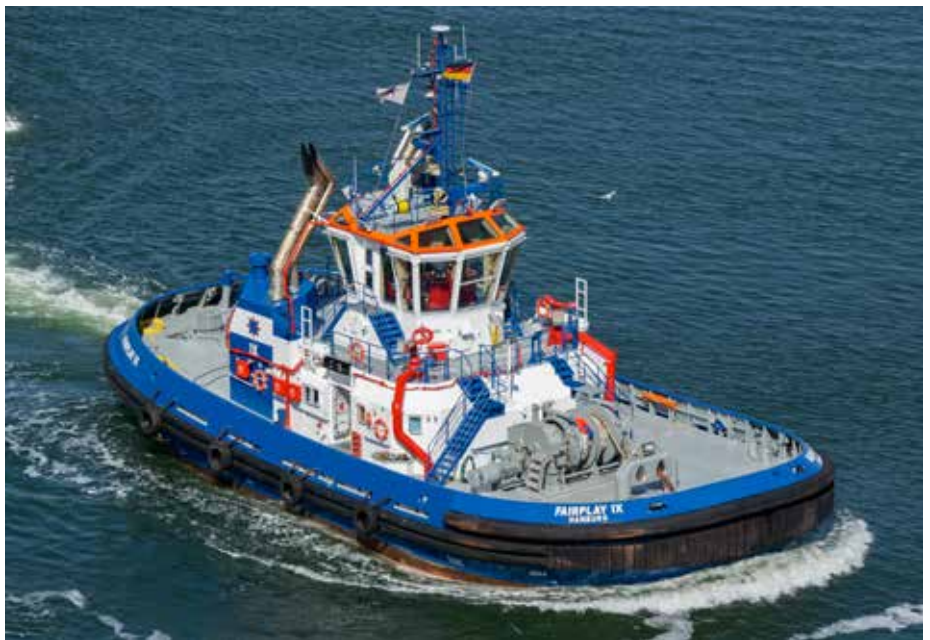
FAIRPLAY IX seen here on 27-04-2015 is fitted with Schottel azimuthing thrusters with hybrid gearbox photo: Hans Hoffmann
