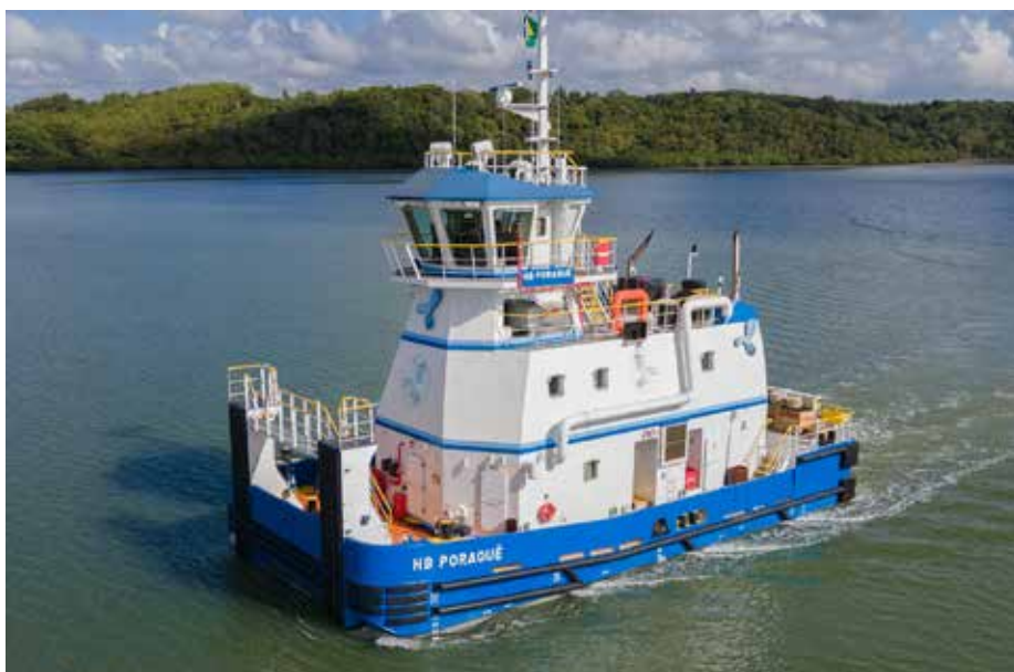
HB PORAQUE is a recently delivered hybrid push boat designed by Robert Allan Ltd for Hidrovias do Brasil. The boat will work on the Amazone River
