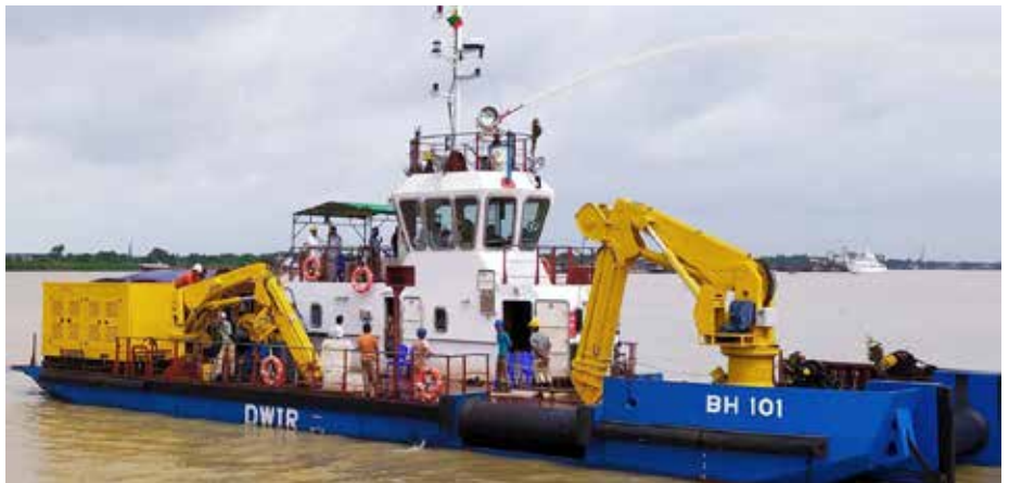
BH 101 buoy-handler with deck-mounted Hydromaster propulsion photo: courtesy Hydromaster
