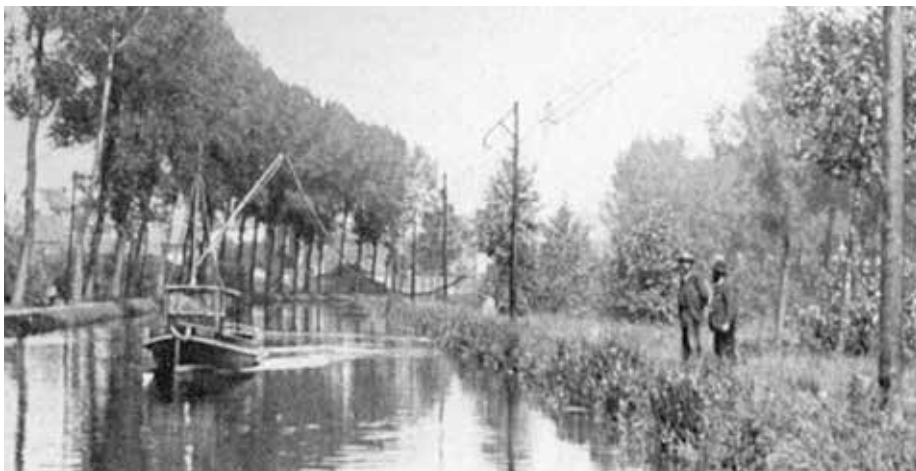
Several 'green'-tugs-avant-la-lettre sailed in Belgium around 1900. They were electric-only being power-supplied through a trolley system photo taken from a 1976 Lekko-publication
