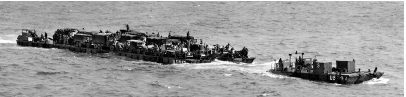
Rhino ferry RHF-3 assisted by Rhino tug RT-3 seen here on 5 June, 1944, approaching the Normandy beaches. This type of propellers were post-war licensed to the U.K. which evolved into Hydromaster photo: U.S. Coastguard (Wiki Commons Public Domain)
