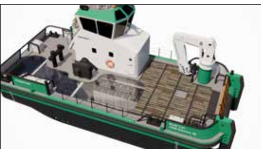
Cut-away rendering showing battery racks artwork: Damen Shipyards
