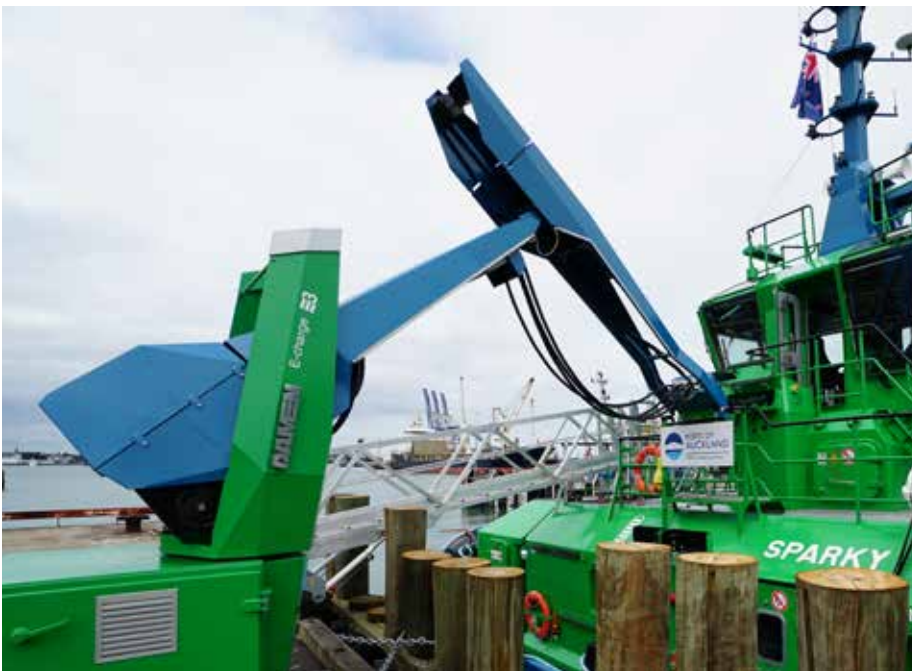
Shore charging station developed by Damen for charging electric tugs photo: Damen Shipyards
