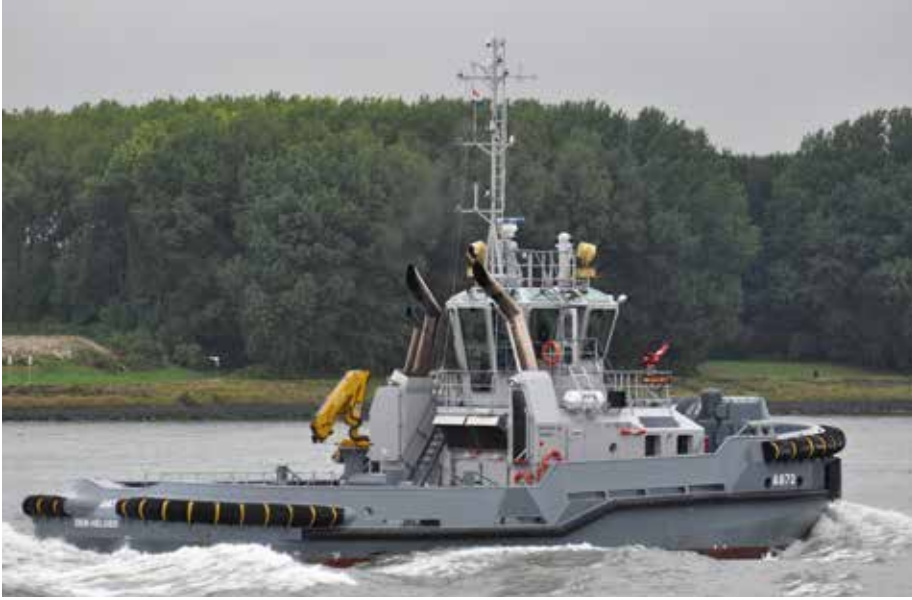
The Dutch Royal Navy acquired three Damen ASD-2810 hybrids. The battery packs are charged via the shore-power plant at the Naval Base, Den Helder. WADDENZEE is seen here 30-08-2017 en route Rotterdam photo: Ruud Zegwaard
