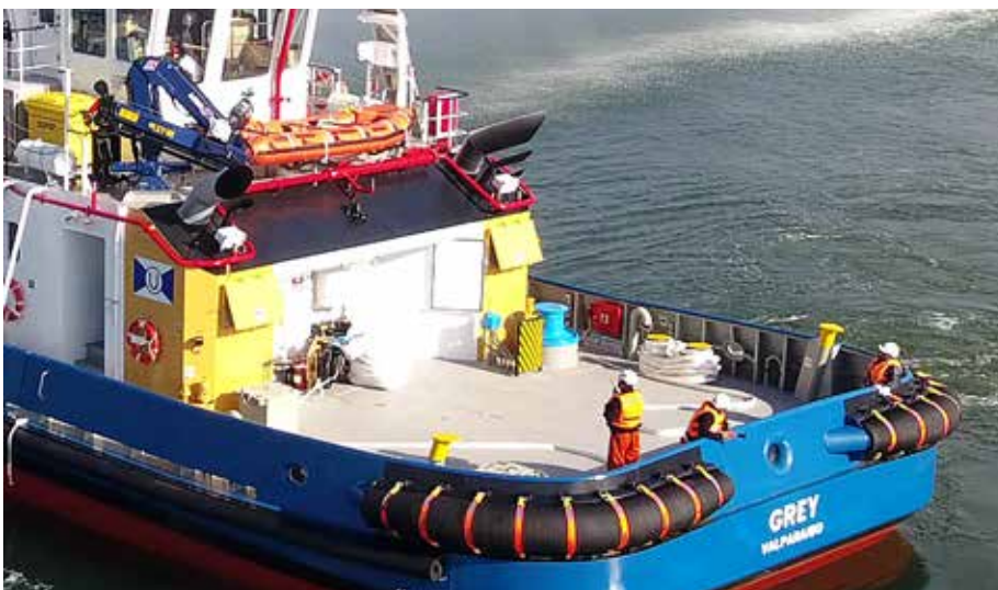
Aft deck - note position of crane and m.o.b. workboat
