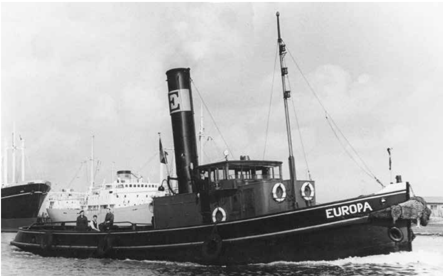
P. Smit Jr.'s EUROPA was built as BANKA in 1916 by the P. Smit shipyard. 25,03 / 23,37 x 6,10 x 2,82 m. Draught 2,60 m. 375 ihp. 1924 renamed EUROPA. Lost seagoing certificate in 1935. Sold for scrap in 1957
