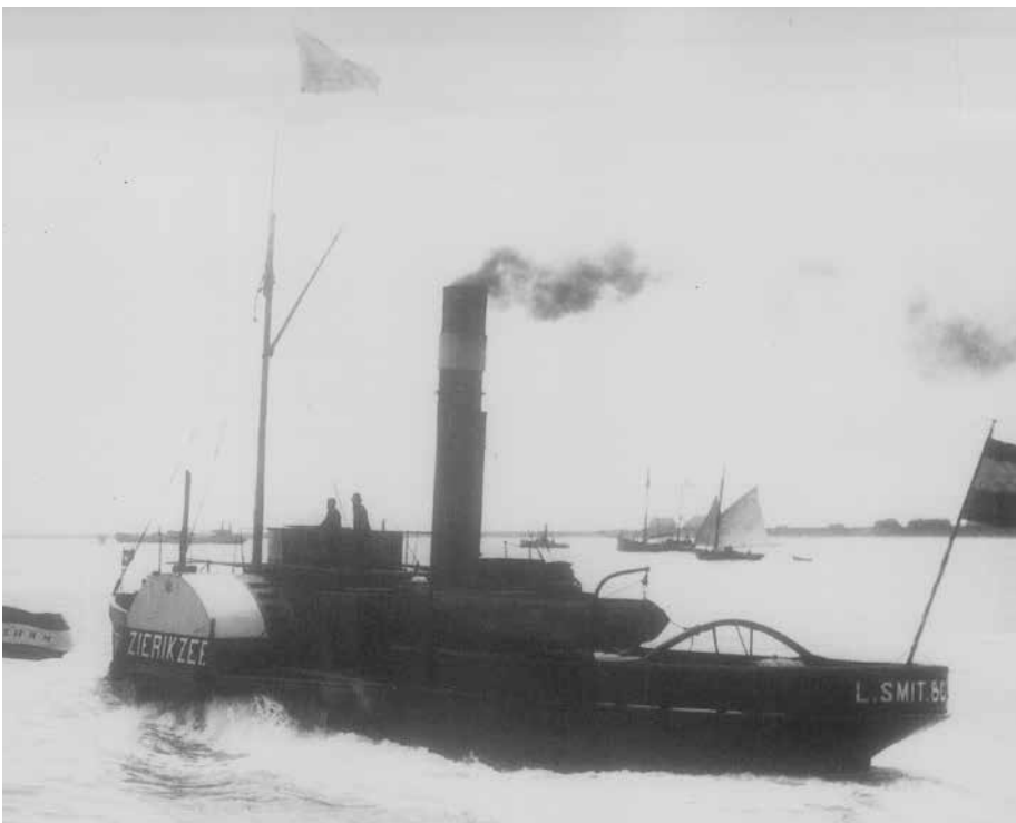
L. Smit & Co.'s paddle tug ZIERIKZEE ex ROTTERDAM I (owner Gallas). Built 1958 by Paul van Vlissingen en Dudok van Heel, Amsterdam. 29,00 (oa) x 11,00 x 2,25 m. Draught 1,90 m. Acquired 1868. 1894 sold for scrap photo: coll. Job van Eijk
