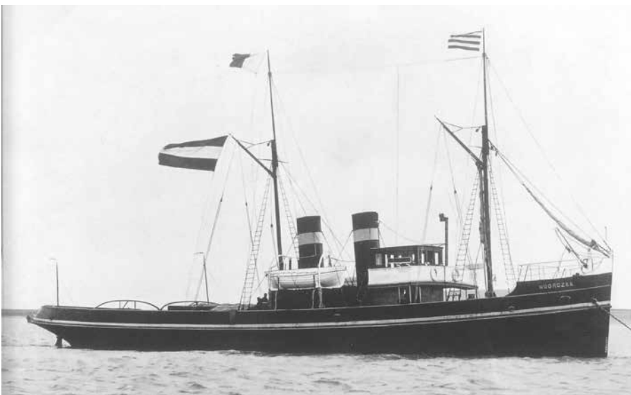
NOORDZEE built in 1892 by L.Smit & Zn Shipyard, Kinderdijk, was the first of two tugs ordered for deepsea work. 39,00 / 37,80 x 7,37 x 3,66 m. Triple expansion steam engine, output 690 ihp. 1909 lengthened to 44,980 m. Second funnel removed. 26 April, 1916, mined near Galloper LV and sunk photo: L. Smit & Zn. Shipyard
