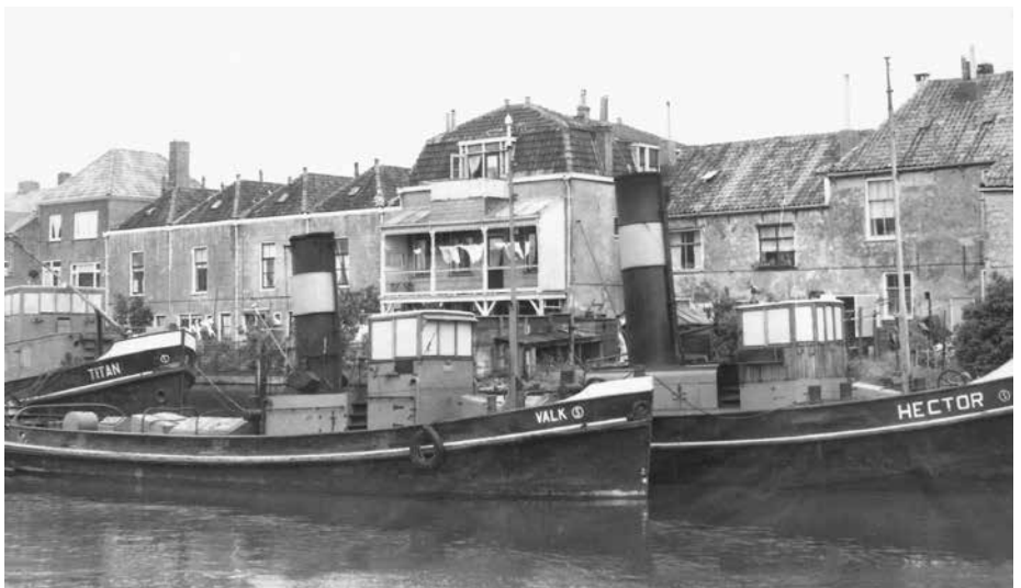
VALK (nearest camera) and HECTOR. L. Smit & Co's Internationale Towagge Co. - Built 1930 resp 1927 by Piet Smit Jr Shipyard. 150 ihp resp 430 ihp. Both sold 1958 to Genoa, Italy photo: Foto Teunissen
