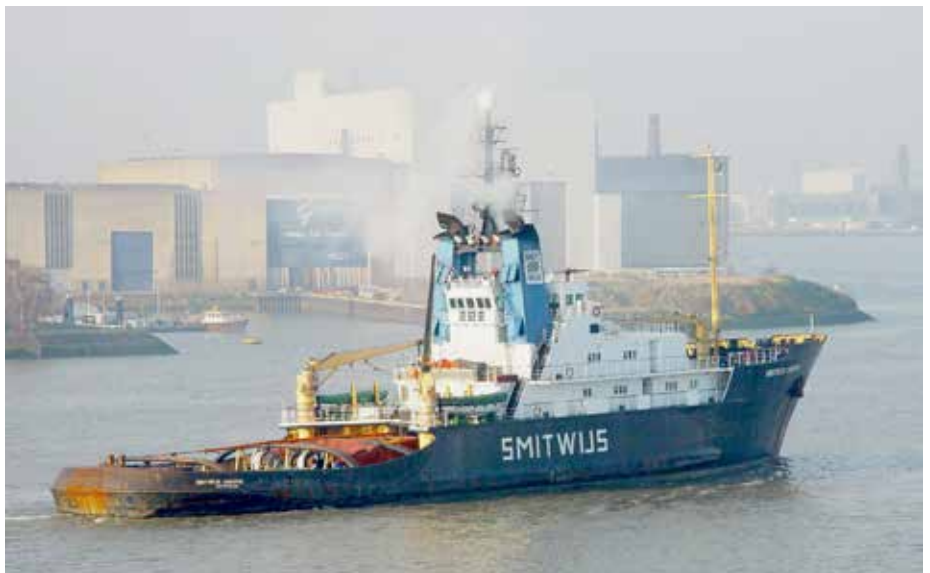
SMIT LONDON - 4th generation Smit ocean tug - seen here already under the SmitWijs banner (since 1991) as SMITWIJS LONDON Bahamas . Later to Svitzer as LONDON and finally scrapped as GLOBAL CHANGE . Built 1975 by De Merwede, Hardinxveld. 74,83 / 66,90 x 15,78 x 7,60 m. Draught 6,80 m. 2x 9-cyl Sork Werkspoor total output 13.500 bhp (marketed as 22.000 hp) photo: Job van Eijk
