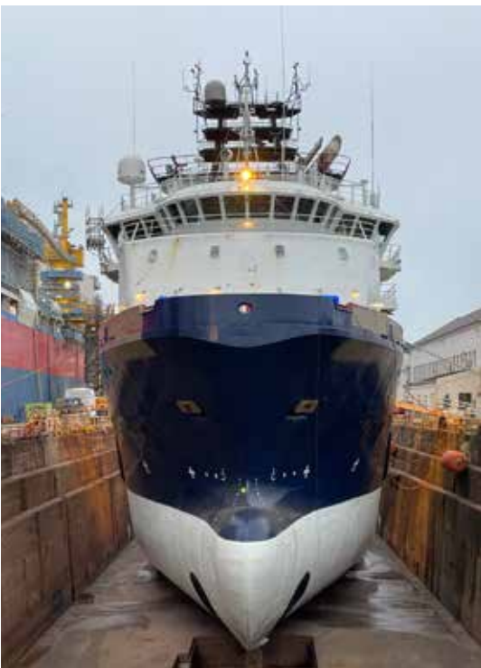
K.J. GARDNER receiving its new hull coating photo: Kotug Canada
