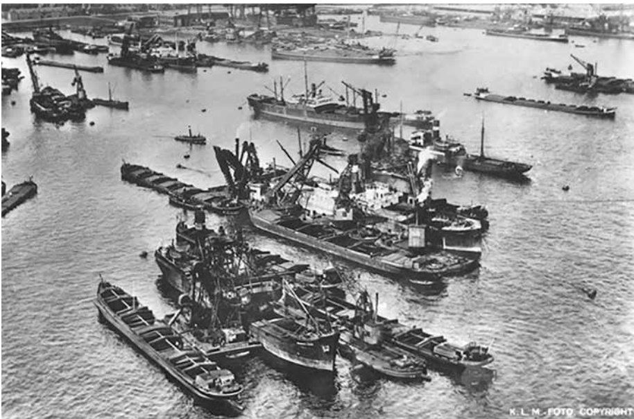
The Scheepvaart en Steenkolen (SSM) site in the Waalhaven. Cargo vessels discharging in resp loading from barges with the use of floating cranes and elevators
