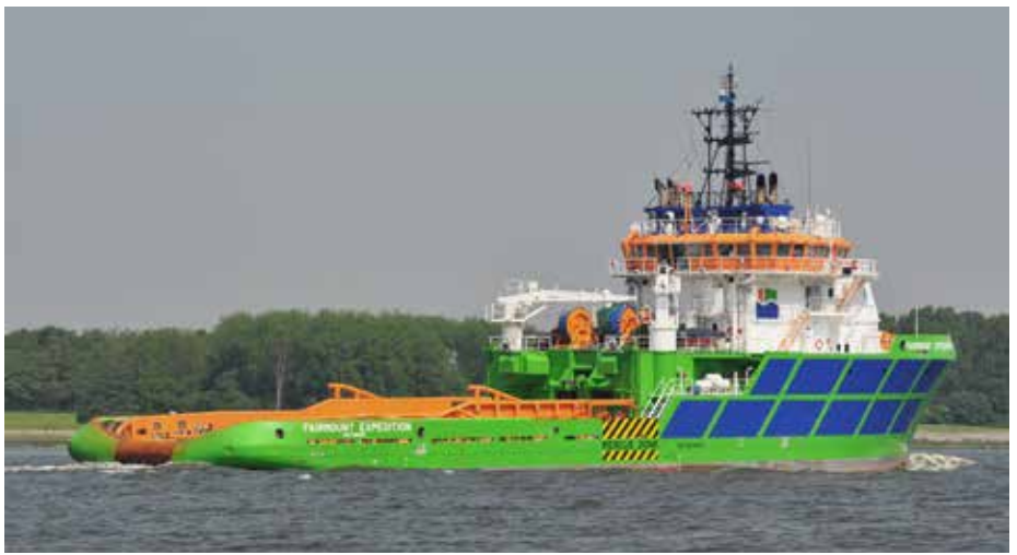
FAIRMOUNT EXPEDITION, on of five 200-tbp ocean tugs built for Henk v/d Berg's Fairmount, then were sold to Louis Dreyfus only to return a few years later to The Netherlands for Boskalis
