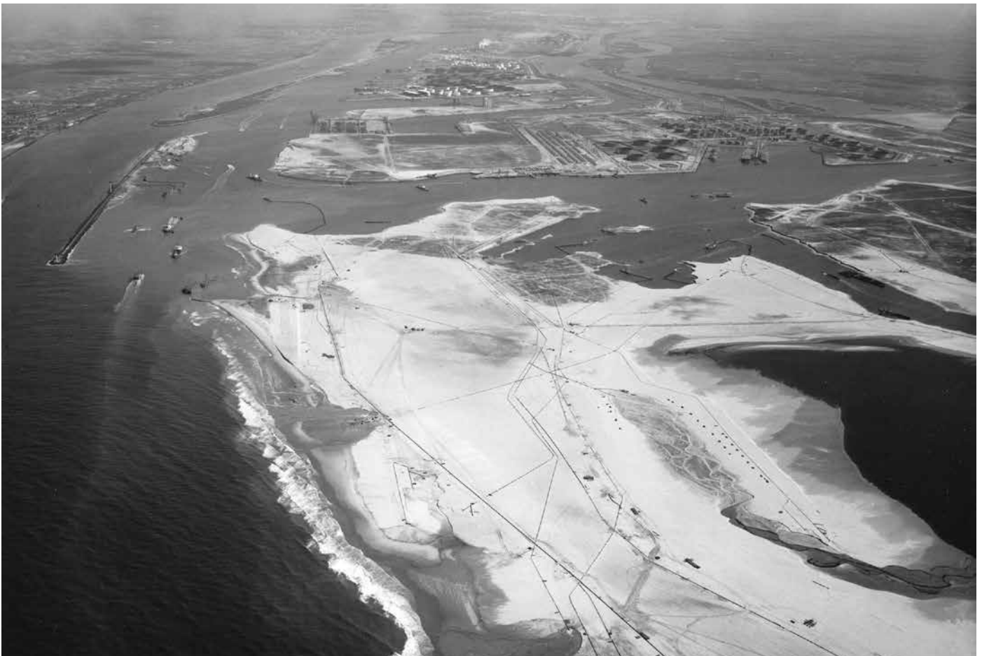
Situation in 1972. On the left the New Rotterdam Waterway, centre the Europoort with on the right the Maasvlakte under construction. The Caland Canal runs parallel to the Waterway with the harbours and the industry on the right. The Beer Canal connects the ports area to the far right with the entrance to Europoort. At the top of the photo is the temporary entrance
