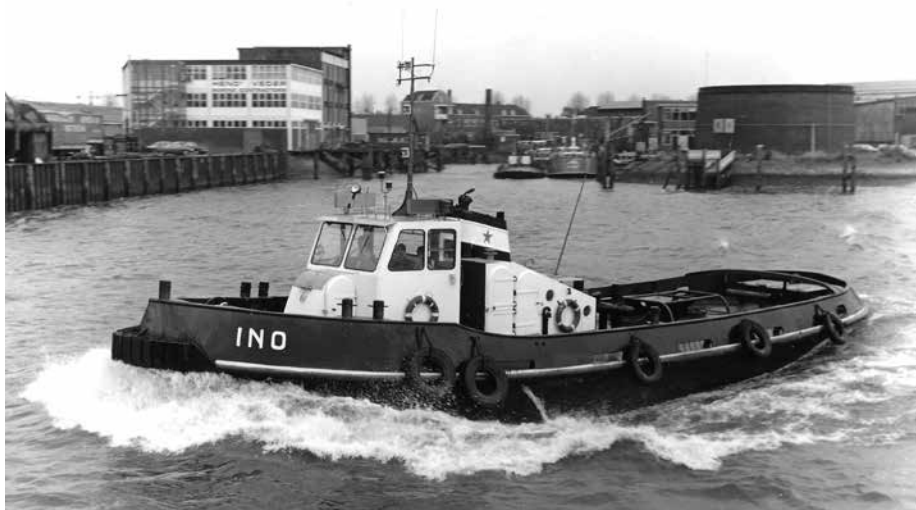
INO in the colours of Hudig & Veder. Built 1952 D.& Joh. Boot - 22,32 x 6,32 x 2,40 m. Industrie diesel 450 bhp - 1986 to Smit International - 1987 sold. This is an example of the smaller type of harbour tug immediately after WW2.
