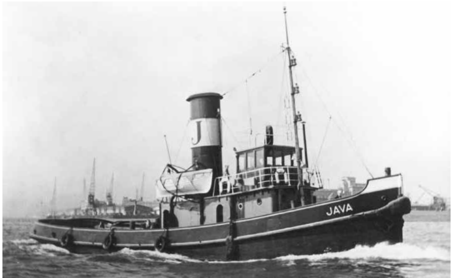
P. Smit's JAVA ex MAAS ex BEATRIX was built in 1918 for Van der Schuyt. 1918 to Internationale Sleepdienst as MAAS. 1936 purchased by P. Smit Jr. Confiscated by Germany during WW 2. 1945 returned. Sold 1952 to Conakry as SAINT ENGRACE. 452 ihp. 30,10 / 28,29 x 6,45 x 3,05 m. Draught 2,85 m photo: coll. Job van Eijk
