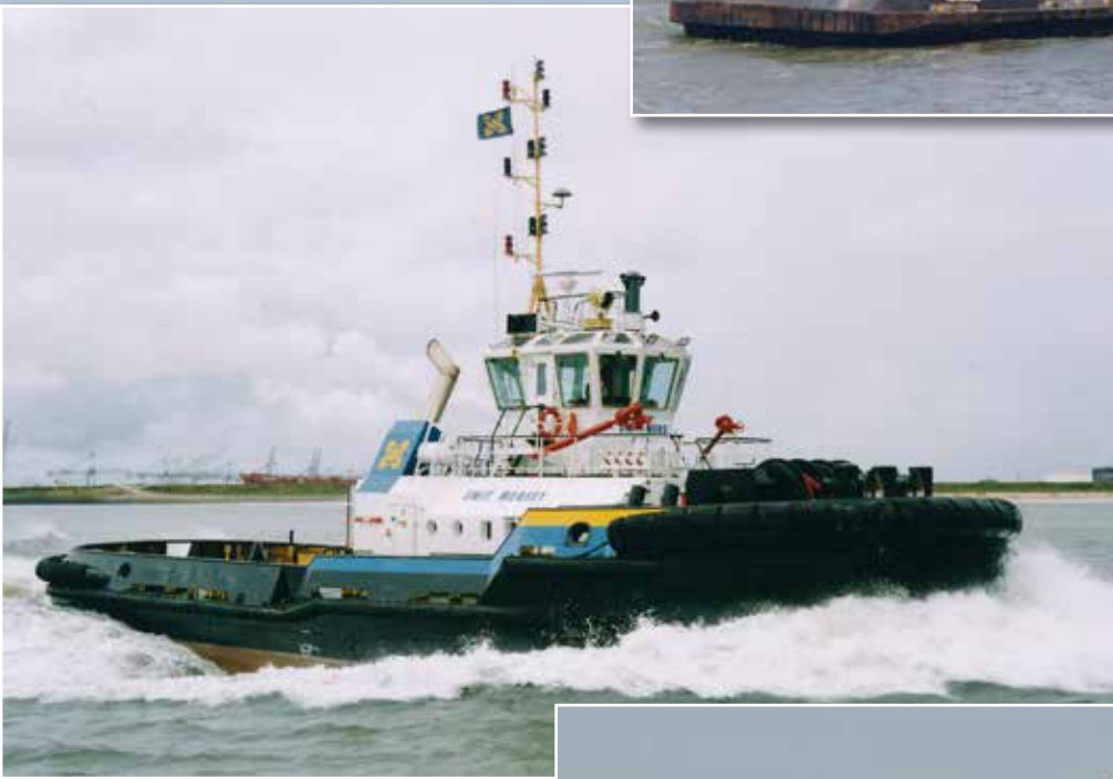
Third generation Rotterdam shiphandling tug: reverse tractor tug designed by Damen Shipyards: SMIT MERSEY built 1999. 4.908 bhp - 61,3 ttp. 2009 renamed SMIT NIDA operating in Lithuania. 2013 to Smit Lamnalco as SL NIDA. 2019 sold to Canada as DALTON WARRIOR. Delivery trip was under the name of IDA 1
