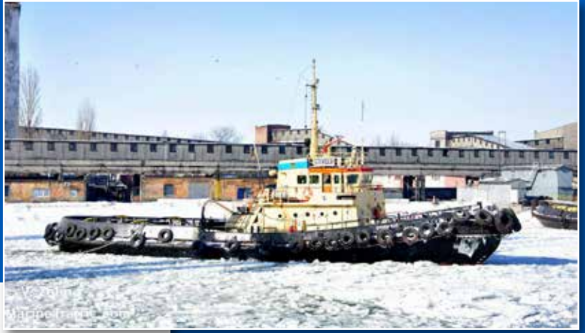
STIVIDOR was built in 1973 by Brodogradiliste Tito. 35,4 x 9,3 x 3,2 m. Main engines 2x B&W total output 2.300 bhp - speed 13,6 knots
