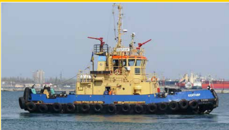
KENTAVR - built 1988 at Brodogradiliste Tito - Main engines 2x MAN total output 816 hp. Owner listed as Odessa Commercial Port
