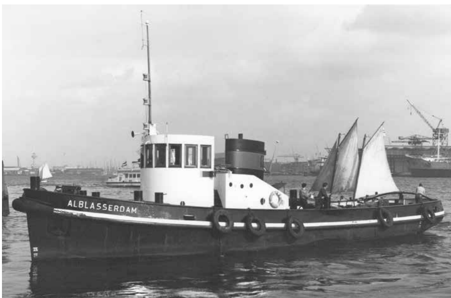
ALBLASSERDAM is the former PERNIS, completed in 1939 by J.& K. Smit for account of L. Smit Internationale. 24,72 / 23,00 x 6,50 x 3,30 m, Draught 2,46 m. Diesel-electric, output 540 ihp. Renamed ALBLASSERDAM in 1955. Prototype for a generation of L. Smit Internationale shiphandling tugs. 1976 reconstructed. 1985 sold as DIKKY to Koehoorn, Harlingen photo: coll. Job van Eijk
