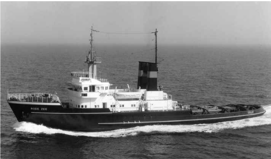
RODE ZEE - 3rd generation Smit ocean tug after WW-2. Built 1968 Arnhemsche Scheepsbouw - single screw 7.000 bhp (11.000 hp) - 68,50 / 65,08 x 12,60 x 6,40 m. Draught 5,65 m. 1987 sold Triple S Marine - 1988 scrapped photo: Skyfotos / Fotoflite
