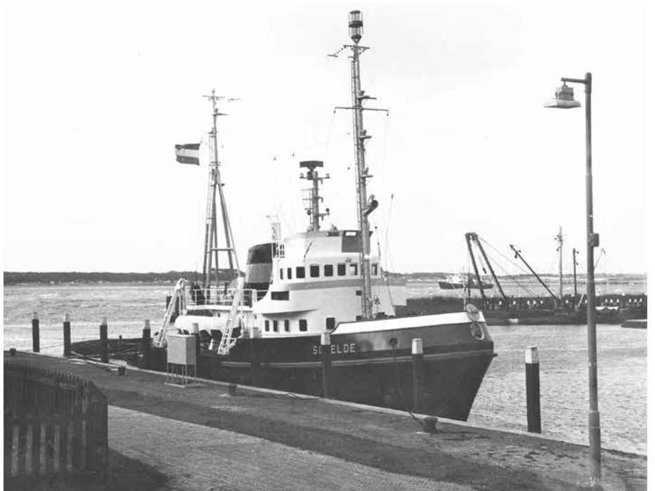
SCHELDE was built by J.& K. Smit in 1959 for Smit's salvage station at Hoek van Holland. 44,63 / 41,89 x 9,47 x 4,09 m. Draught 3,08 m. Diesel-electric 1.800 bhp. 1967 re-engined with 3x Kromhout, total output 2.250 bhp. 1970 transferred to Smit Antilles. 1976 sold or transferred to Holyhead Towig as AFON GOCH . 1980 GOLDEN VENTURE , 1983 CORWIN , 1986 NOBLE VENTURER , 1987 TX TX STAR . 1990 burned at Houston, total loss photo: coll. Job van Eijk
