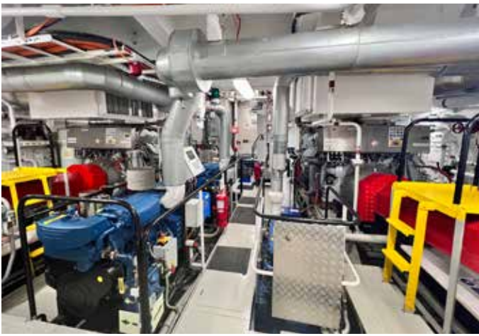
Engine room looking forward with gen sets (left) and harbour set sitting between the main engines
