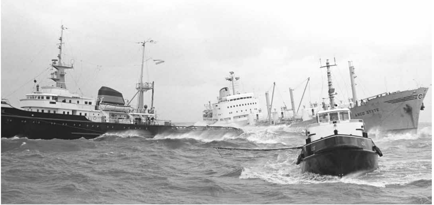
Salvage action at Hoek van Holland - the NRS Voith Tractor AZIE holding the bow (no bowthrusters then) of the brand-new WITTE ZEE (9.000 ihp) - still flying the shipyard flag - as she is backing down to connect to the bow of the laden chemical tanker ANCO STATE stranded on the North Mole at Hoek van Holland in seriously bad weather. Sister ZWARTE ZEE was also on the spot. The tanker, however, was unable to get the heavy towing wire on board. Later refloated by a fleet of NRS tugs. The reason for the use of the muscle was that a spill of the tanker's cargo could have had serious consequences for the people of Hoek van Holland, just 3 kilometres away photo: Rotterdam City Archives
