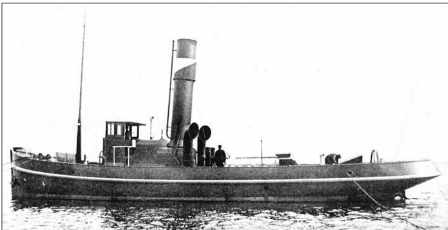
The steam tug HIBERNIA was built in 1911 by the Gusto Shipyard for account of the SHV. 22,50 x 6,00 x 3,00 m. 400 ihp. Sold 1916 to the Corinth Canal Company, Piraeus, as ELLIE
